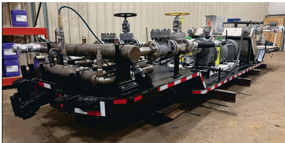
Pumps can be mounted on railcars to accompany cutting machines.
