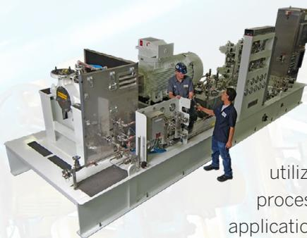
Built to API-617 standards, the Sundyne BMC (Base Mounted Compressor) product line features horizontal single-stage integrally geared centrifugal designs that process engineers utilize for midstream, hydrocarbon processing and chemical manufacturing applications. These horizontally-configured compressors are ideal for skid packaging, due to their unique modular baseplate and are designed to run continuously for 5 years without costly maintenance.
