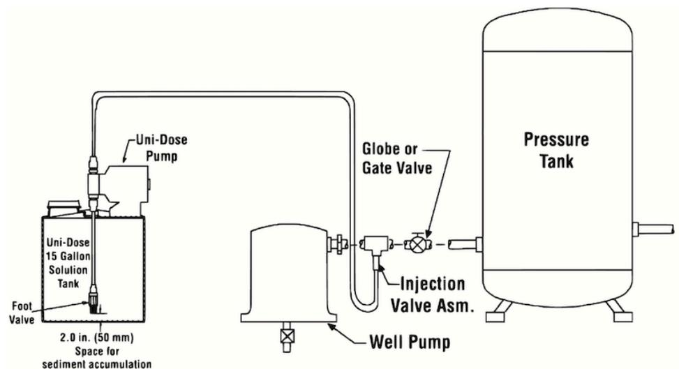
in the process is the critical point-of failure for the entire system—so the liquid end of the metering pump must be constructed of materials that can withstand these harsh chemicals for years.
